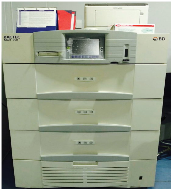
Figure 3: Bactec MGIT 960 (Automated liquid culture equipment).
