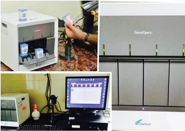
Figure 2: Gene Xpert equipment with cartridges, monitor and scanner for CBNAAT.
